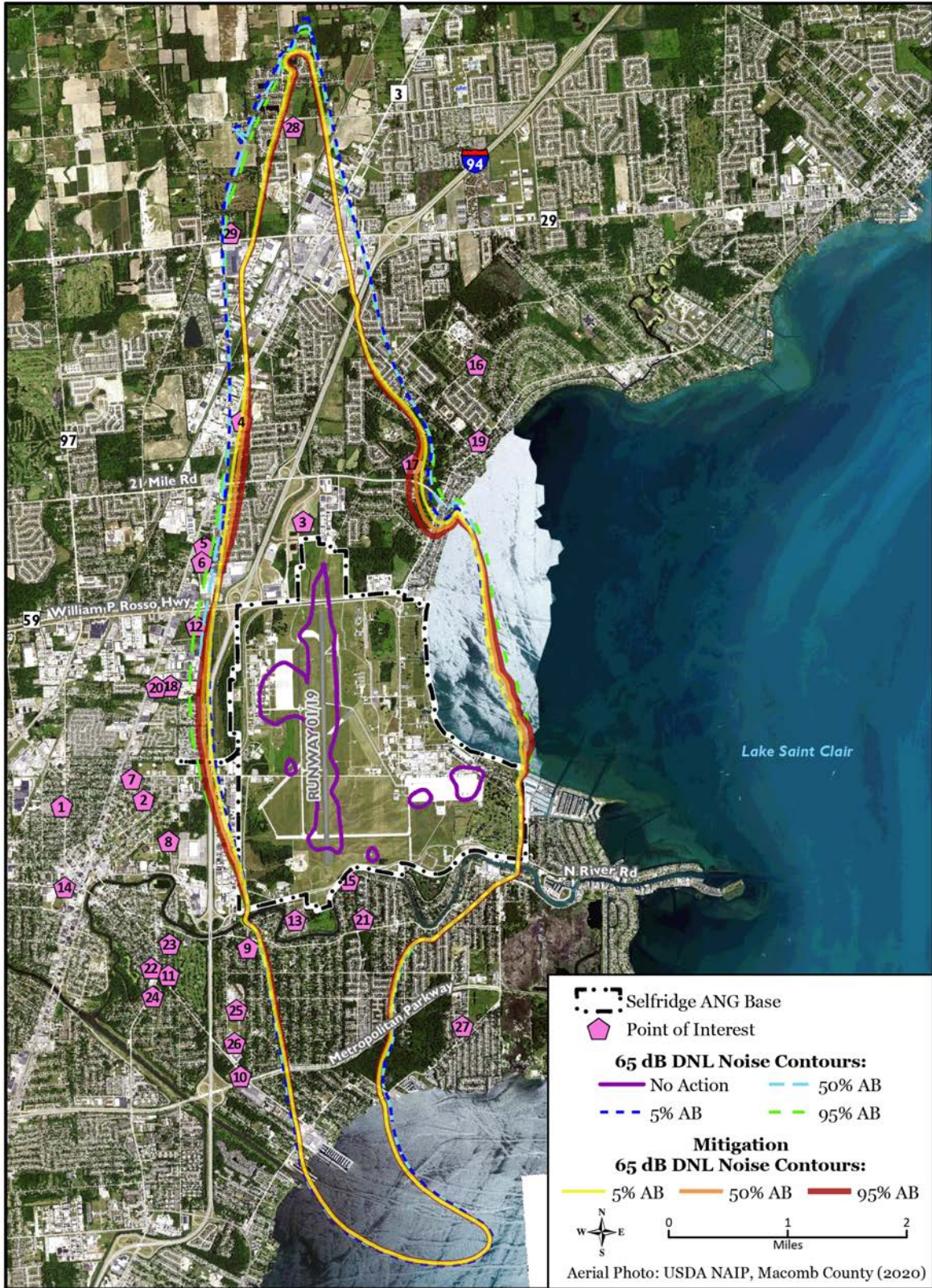
Figure 4.3-8. Comparison of 65 dB DNL Noise Contours for Mitigated and Original Operations Under Preferred Alternative F-35 Afterburner Use Scenario Near Selfridge ANG Base
